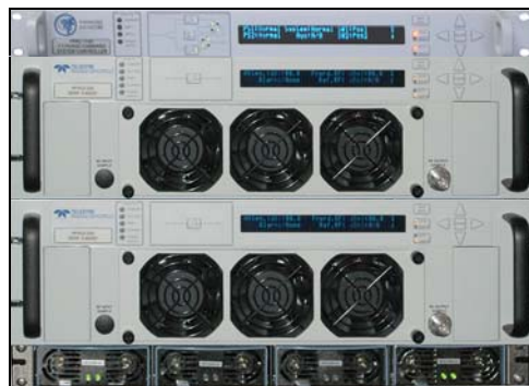
◀ 300W C-Band (3RU) 1:1 Phase Combined System
