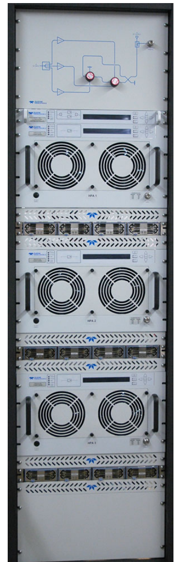
2kW C-Band (6RU) ▶ Phase Combined SSPA System
