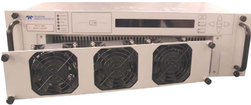
Removable front panel fan tray
