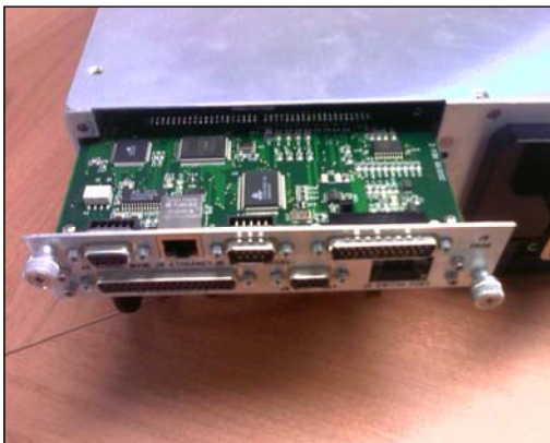
Removable rear panel monitor and control card
