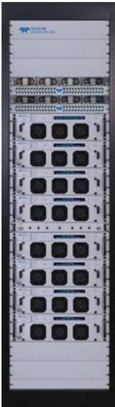
PowerMAX System with 8 SSPA Modules
